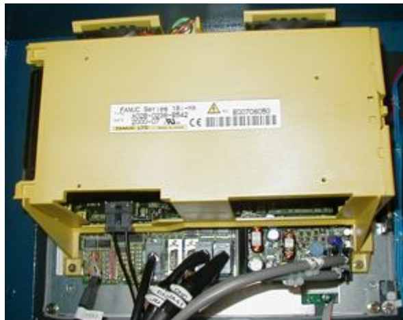
A Fanuc 18i Model A Control From Behind The Monitor
